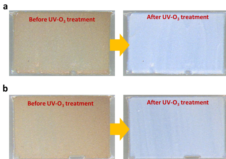
Fig. S2. Photographic images of the 150°C sintered TiO 2 films prepared using (a) P BL and (b) P O before and after UV-O 3 treatment.
